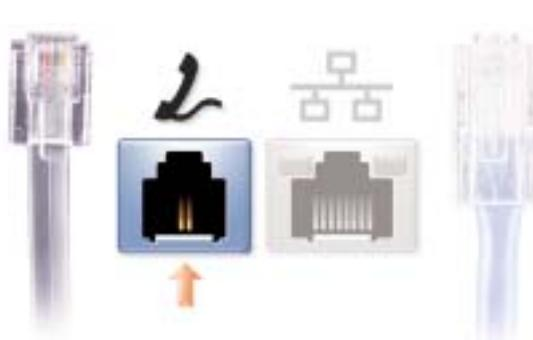
If your computer has an internal modem, connect the telephone cable to the modem connector and connect the other end of the cable to a telephone wall jack.
