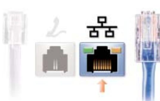
If your computer has a networking option, connect a separately purchased network cable to the network connector.
